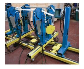
Unique to Rotary is the Coil Jig, developed with the UK's top coil makers, this new piece of equipment enables you to check the geometry of a coil without the need to manufacture a coil former for each design you produce. In addition, the jig is sufficiently robust to allow for final coil shaping in situ if required. The Coil Jig also features location points for customers own coordinate measuring equipment, allowing precise inspection of the finished coil geometry.
