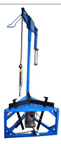
The coil puller, designed and made by Rotary, is designed to remove faulty coils from electric motors which require rewinding. When the coil end has been cut off (using a stator cut off machine), the stator is turned on its end and then secured on the coil puller for the extraction operation. Using this equipment greatly reduces the risk of damaging the core pack / laminations.
